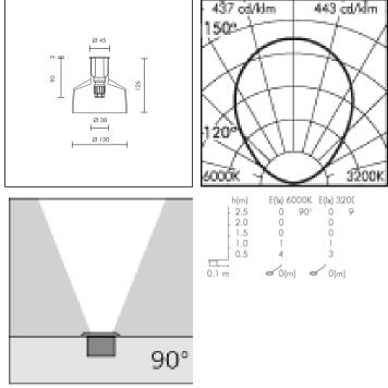
\*Photometric measured using COLD WHITE LED 6650K
