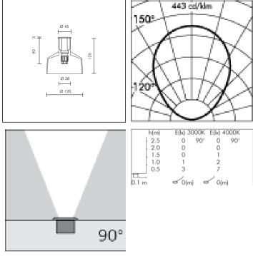
\*Photometric measured using COLD WHITE LED  $6650 \mathrm{K}$
